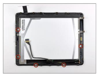
• Remove the remaining T4 Torx screws securing the LCD to the black plastic display frame.
