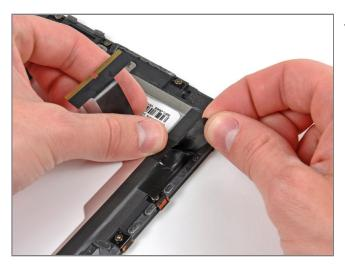
While holding the digitizer cable down, carefully peel back the piece of tape connecting the digitizer cable to the display frame.
