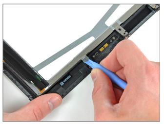
Repeat the process detailed on the previous step to pry up the display around the three sides opposite the digitizer cable side of the display.
